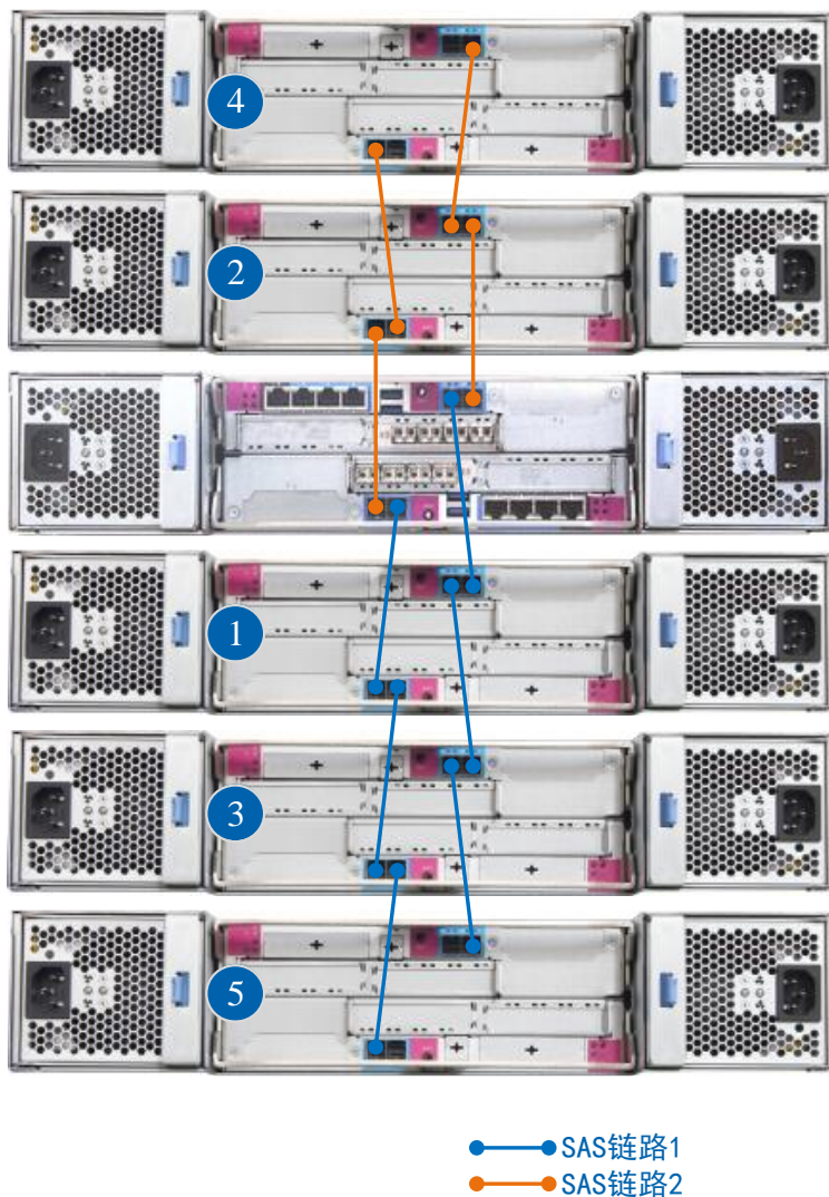
图 3-4 连接 5 台扩展柜-AS2150G2&amp;AS2200G2&amp;AS2600G2&amp;AS5300G2&amp;AS5500G2
